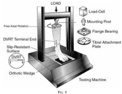
Illustration of the *in vitro* test setup. DVRT = differential variable reluctance transducer.
