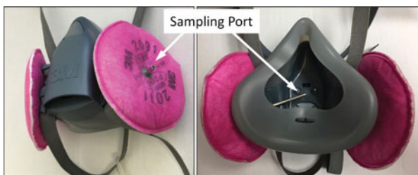
Figure 1. 3M 3500 series respirator probed for fit test with stainless steel sampling port extending to center of mask.
